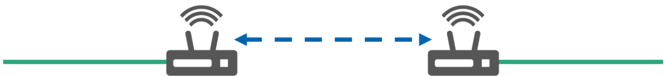
Figure 5 - Point to Point wireless topology
