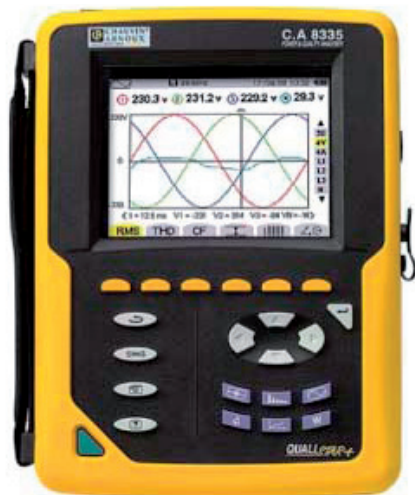
Energy meter used during the audit
